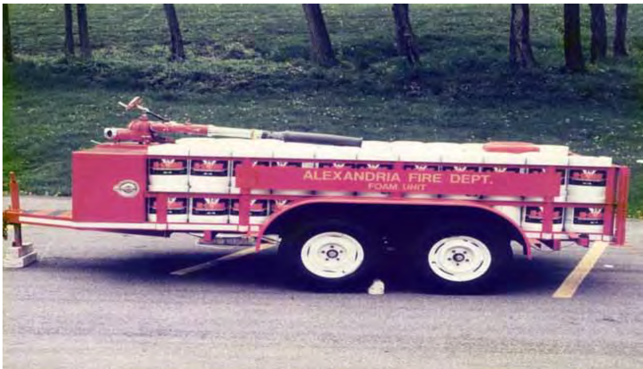
Foam Unit Unit 136 75-5 gallon buckets of foam
